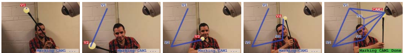
Fig. 4. Progressive capture and marking of veillance field, in order to set up the game and begin the AR experience of veillance. This figure illustrates a methodology to create vector renderings of the veillance field border, as opposed to our other methods that display a raster abakograph of veillance flux.
