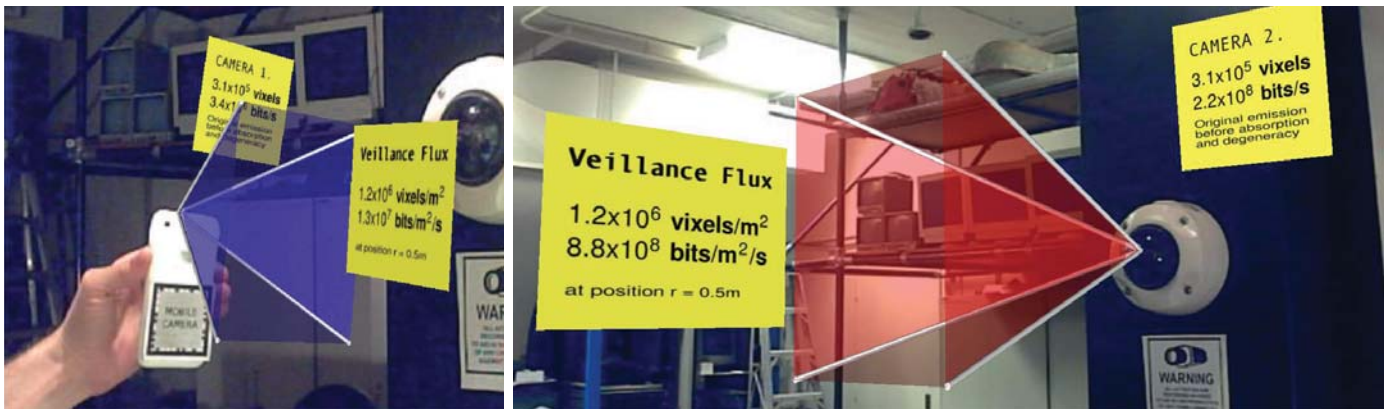
Fig. 3. Real-time augmented reality to see veillance flux, where the system is overlaying statistics about veillance flux from two different cameras.
