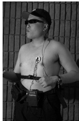
Fig. 1. The wearable HI-Cam as worn by a participant while jogging. Biofeedback is through the viewfinder computer screen included in the EyeTap camera system of the sunglasses.
