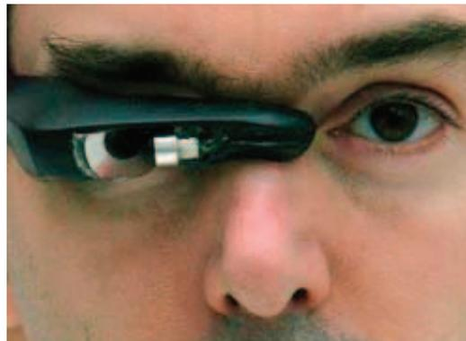
Figure 3. EyeTap visual prosthetic worn by Steve Mann, where the camera-in-the-eye appearance makes use of the fact that rays of eyeward-bound light are diverted into a camera (actually mounted on the nose bridge and pointing toward the wearer's right eye).
