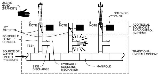
**Fig. 2: Solenoid valves added to a traditional hydraulophone to make it into a player-hydraulophone:** The hydraulophone works like a “player-piano” and plays a portion of a song. Here it is shown playing one note (D). It does this by closing the valve associated with the D note, which diverts water to the hydraulic sounding mechanism. To the user, it appears as if a hidden player is blocking that one jet to make it sound.
