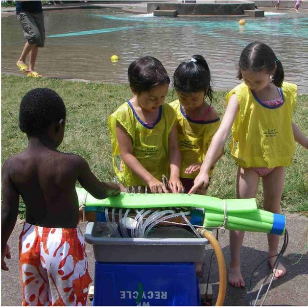
**Fig. 1: Aquatic “Simon” game:** Computer-controlled educational version of a hydraulophone, in which the user interacts with water jets. “Simon” demonstrates how a musical melody is played, by adjusting water flow through the jets. Users who can repeat the melody by covering or diverting the correct water jets are rewarded, and move on to the next level of difficulty. If a user makes a mistake, a buzzer sounds.
