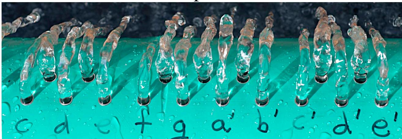
88 spray jets each provide rich tactile/haptic control for one note on the keyboard. Each note sounds different depending on how you press (from above, versus from one side, the top, etc.).
