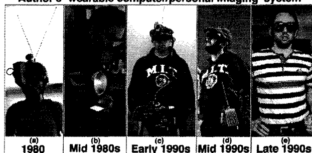
Figure 1: Evolution of author's wearable computer/personal imaging invention. Large head-mounted CRT and separate inbound and outbound communications antennas of the late 70s were awkward. Author's waist-mounted television of the mid 80s was somewhat more comfortable but not constantly visible. Small viewfinders from consumer video cameras of the late 80s made possible an eyeglass-based system which later evolved toward author's current embodiment built into ordinary eyeglasses.
