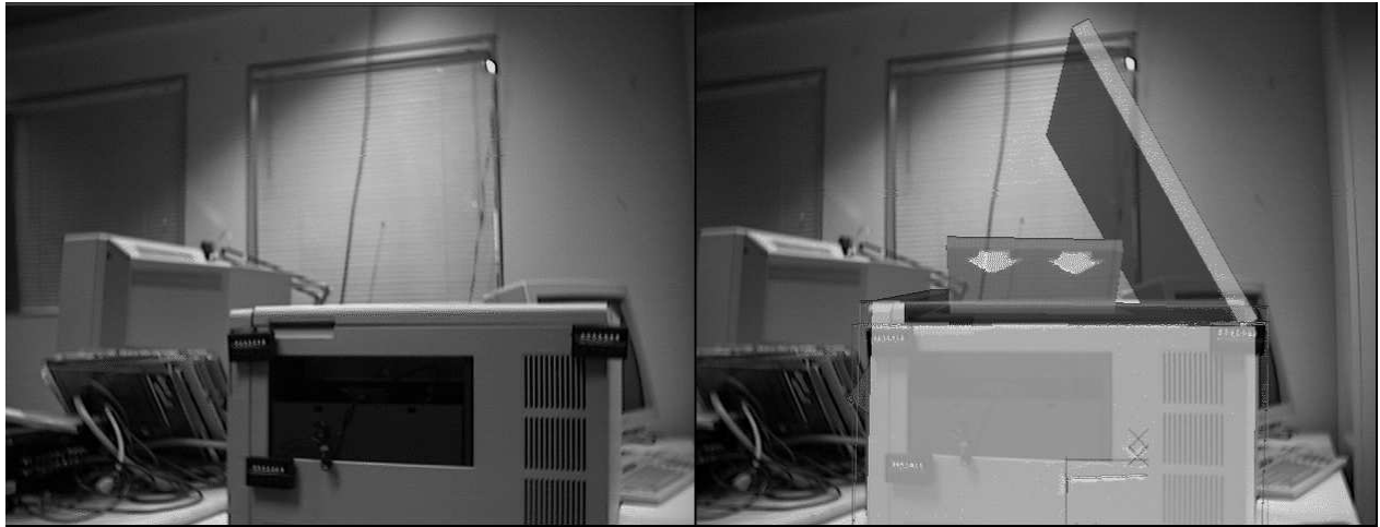
Figure 10: A maintenance task using 3D animated graphics. The left side shows the laser printer to be repaired. The right side shows the same printer with the overlying transparent instructions showing how to reach the toner cartridge.
