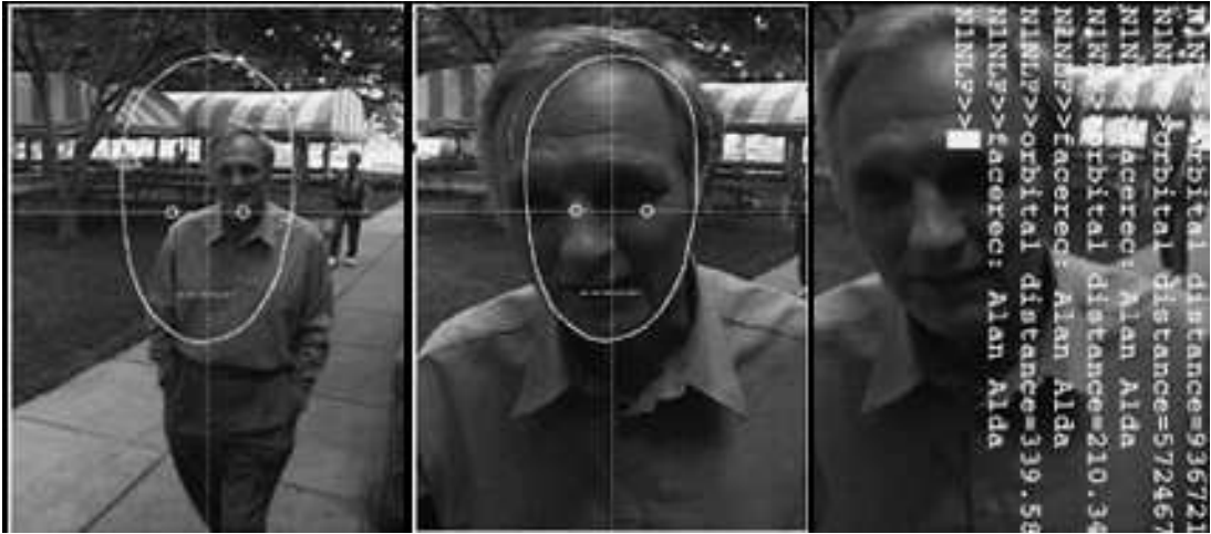
Figure 11: Upon correct identification by face recognition, information about the conversant can be overlaid on the visual field.
