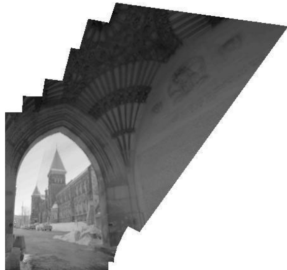
Figure 10: Cemented video frames of Fig 1 after being spatiotally aligned, are now displayed on a logarithmic Quantimetric scale, Q . Here the entire dynamic range is visible, but the image lacks the pleasing effect of high contrast, which we often desire in images.
