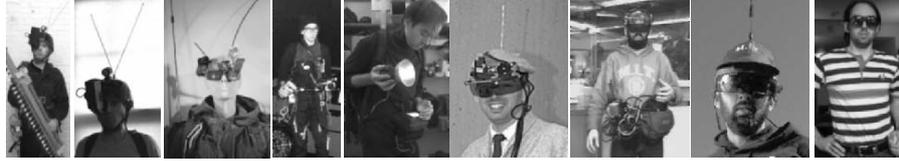
Figure 3. Evolution of the apparatus of the 'WearComp' invention from the 1970s to the present-day version built in ordinary-looking eyeglasses.
