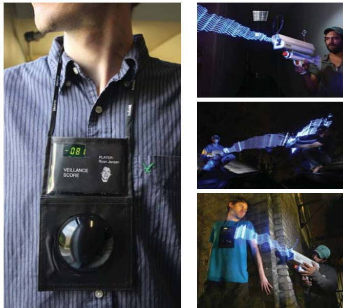
Fig. 6. (LEFT) Veillance Dosimeter. This unit is configured for scopophobic mode: negative numbers accumulate during exposure to veillance flux. The numerical dose reading is scaled down from the raw integral of \nabla , proportionally, to fit within three digits of text. An attenuated dome provides space for optics to sense external veillance, plus optionally an additional camera, for individuals who “emit” veillance flux, i.e. who shoot video of others. (We thank Pete Scourboutakos for aid in arranging the electronics to fit inside the neckstrap pouch, and thank Laura Bolt as test subject in Fig. 5g-h.) (RIGHT) Veillance flux “shot” from a camera: Pulling the trigger causes the camera to “shoot” a picture. The middle image shows veillance flux being reflected by a mirror, while in the lower image, the ability to see is nearly striking an individual’s body-worn dosimeter. Veillance flux was made visible in these photos by combining veillametrics [1] with long-exposure abakography [4] using a video bug sweeper.
