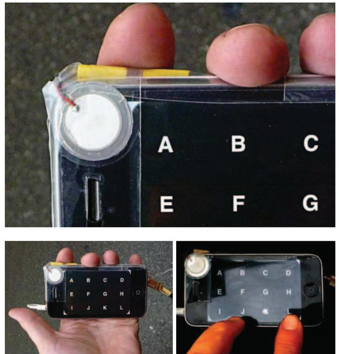
Fig. 5. SqueaKEYs running on an iPhone 3GS. A geophone picks up mechanical vibrations in the solid matter of the screen. There are 12 regions on the screen that can be touched, rubbed, tapped on, or squeezed in various ways. Tapping, rubbing, or the like, on region A results in having whatever acoustic disturbance is created being shifted to 220Hz. Interacting in region "B" shifts to 246.94Hz, in region "C" to 261.63Hz, and so on.
