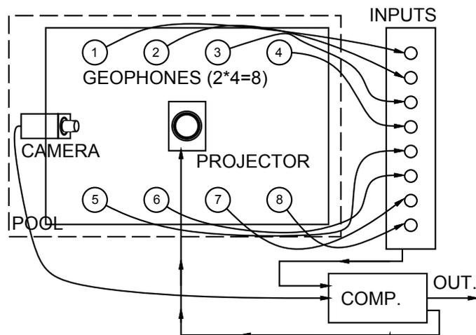
Fig. 4. SqueaKEYs: A continuous friction idiophone as a user-interface. Two linear arrays, each comprising of 4 geophones bonded to the glass surface perform sound localization. A camera provides additional localization, and, though not essential, helps improve the accuracy. A projector completes the touch screen.
