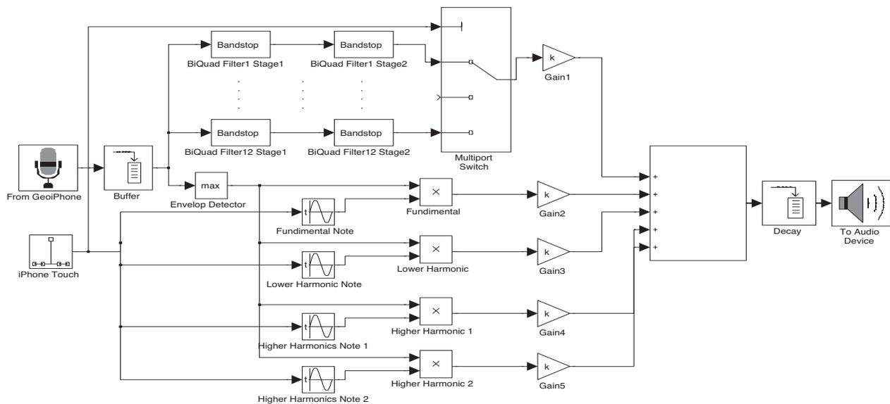
Fig. 6. Frequency shifting algorithm, modifying acoustic content from vibrations of physical tactile interaction. Position-derived control signals allow more control, and act on the original sound simply like an effects processor. This implementation was designed in MathWorks Simulink.
