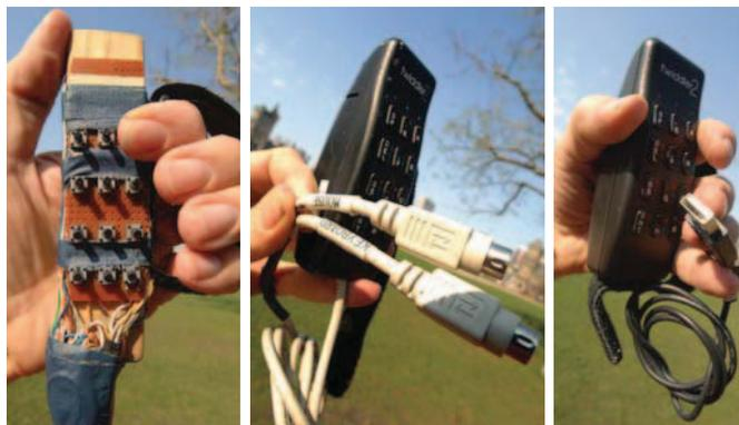
Fig. 1. Examples of handheld keyers with solid keys: Early prototype built by authors; commercially manufactured PS/2 and USB Twiddler keyers.
