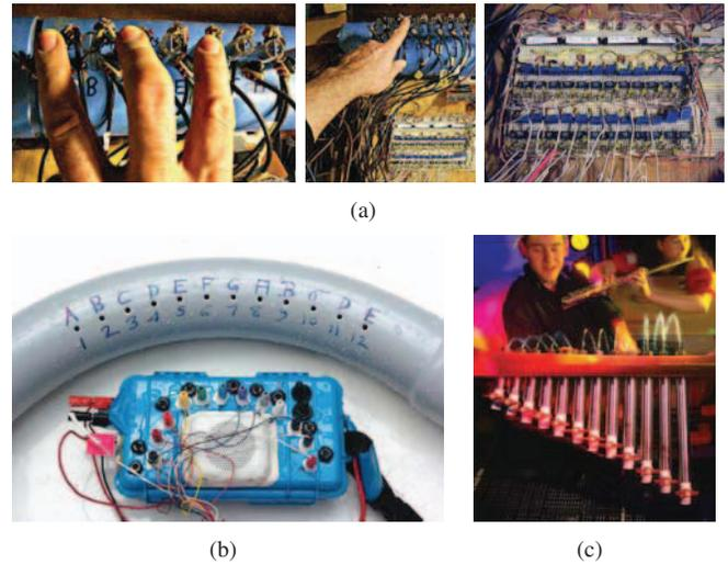
Fig. 2. (a), Instrumented hydraulophone, with 12 channels of dual amplification for bench tests. (b), Instrumented hydraulophone with wearable computer in an underwater enclosure, with waterproof connectors for each of the 12 audio inputs. Compare to an acoustic hydraulophone (c). Musicians use hydraulophones as part of original music performances and compositions, because of their rich expressivity.
