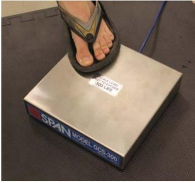
Fig. 3. GCS300 gas cylinder load cell, providing a continuous-time signal from standing, jumping, and a variety of motions. The purpose of the gas is to distribute pressure for equal sensitivity at all points on the top surface. This device which ordinarily measures static weight, we repurpose to measure dynamic motion, and we convert the signal into *actergy* (time-integrated energy).
