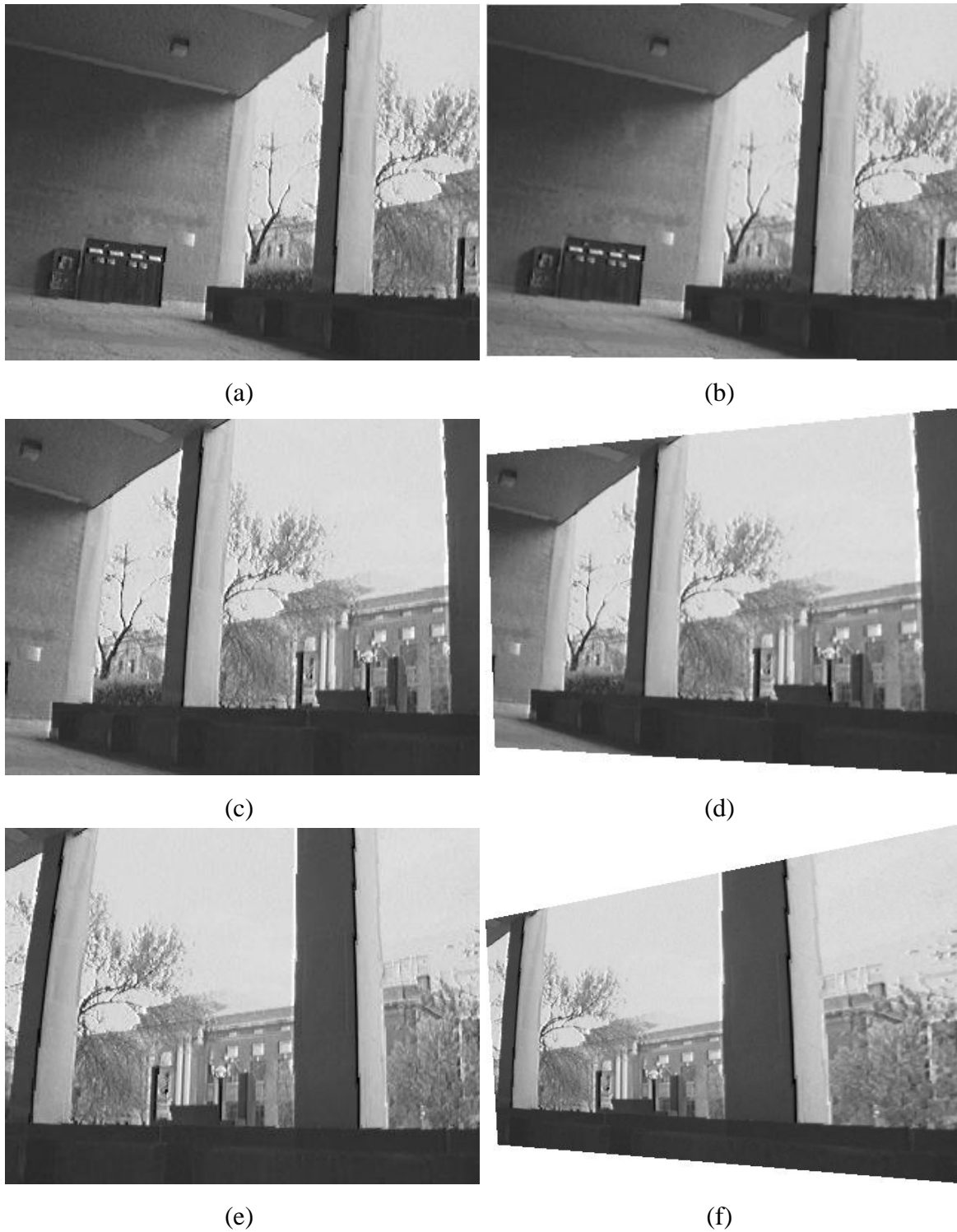
Figure 5.1: (a)(c)(e): Frames of video from an EyeTap device. (b)(d)(f): Images that have undergone a projective coordinate transform to match the perspective of (a).
