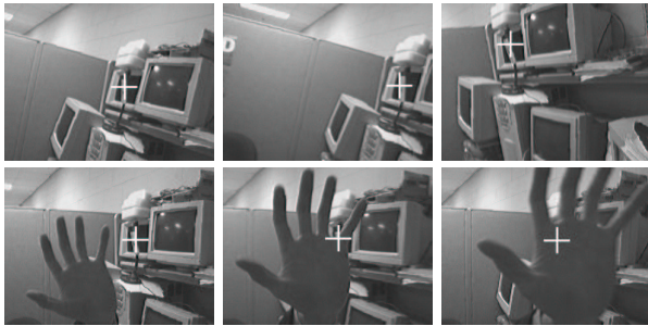
Figure 7: The following images show the GVS tracking a point with significant head rotation in a near environment. The images containing the hand, demonstrate the system's ability to track even when blocked by a large independently moving object.
