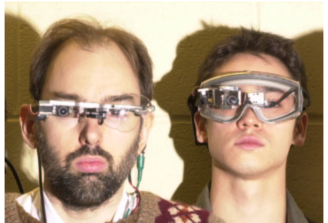
Figure 1: Two examples of EyeTap devices that tap the right eye. Note that both eyes can be tapped if stereo computer mediated reality is desired.
